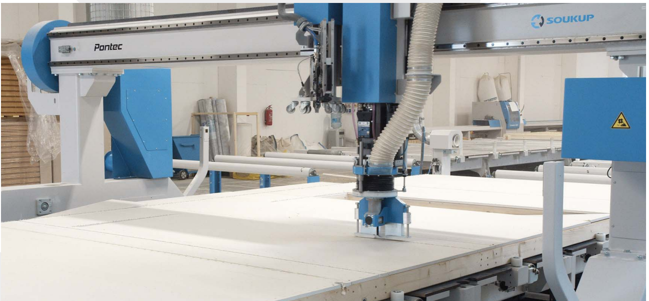
Saw unit with integrated extraction
