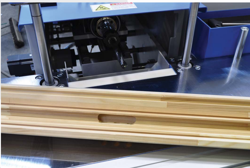
Longitudinal milling and drilling
