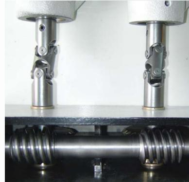
Highly precise feeding system with worm gears and cardan drives
