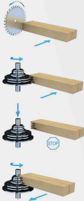
Tenoning machine with a forwards-backwards working cycle
