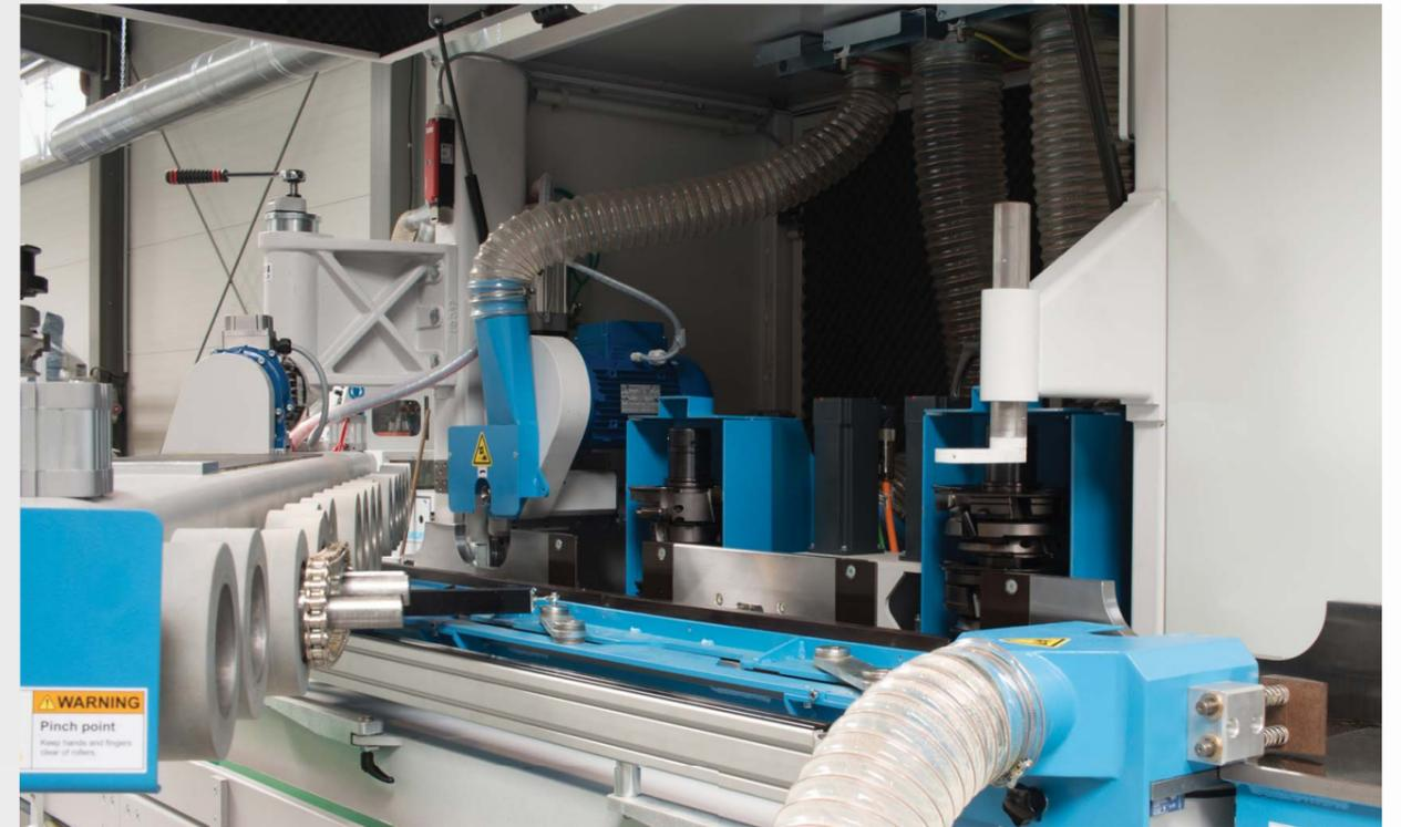
Profiling machine for complete moulding of timbers in one single operation
