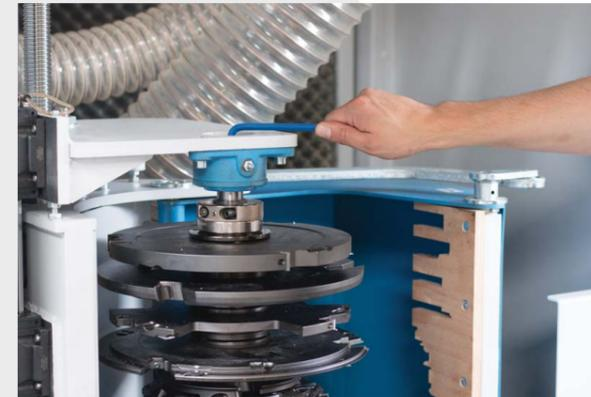
release shaft bearing using allen key
