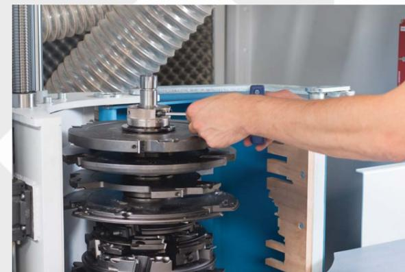
release hydro nut using allen key
