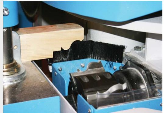
Horizontal milling unit for horns and trenching operations
