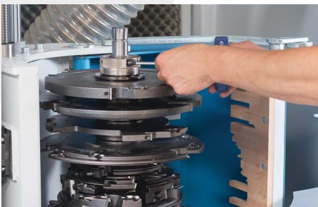
Tenoning with a forwards-backwards working cycle
