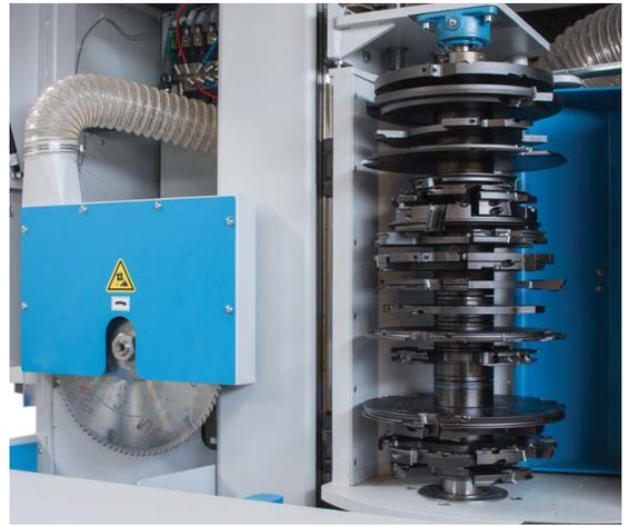
Another member of the Wizard family is the [Wizard 3S](#). This machine is designed for the production of traditional windows (which commonly have complicated profiles) or, often, alu-clad windows. The machine offers absolute durability, full electronic control, extra space for tooling and everything that you would expect from an industrial machine.
